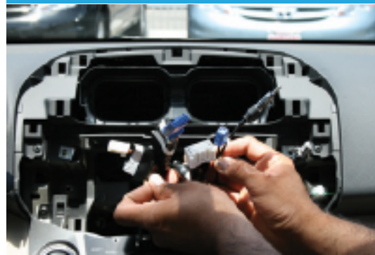
Step 2. Locate all the factory wires
