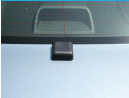
Step 1. Mount GPS and Satellite radio antenna
